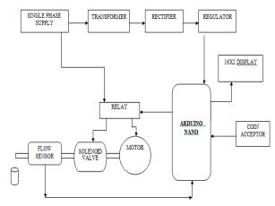
Fig. 1: Block Diagram
