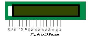
These modules are preferred over seven segments and other multi segment LEDs. The reasons being: LCDs are economical; easily programmable; have no limitation of displaying special & even custom characters (unlike in seven segments), animations and so on.
